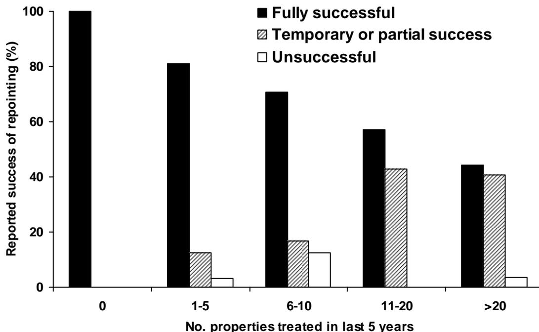
Figure 1.16 The influence of level of experience on practitioners' reported success with respect to repairing major physical defects as a treatment for damp penetration. This combines reported results of repairs to slates, tiling, tilted fillet, skews, gutters and downpipes.
