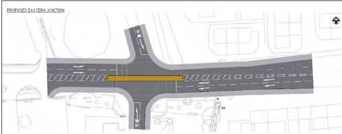
Fig 24 – Eastern Junction – indicative layout – final left-in/left-out solution
