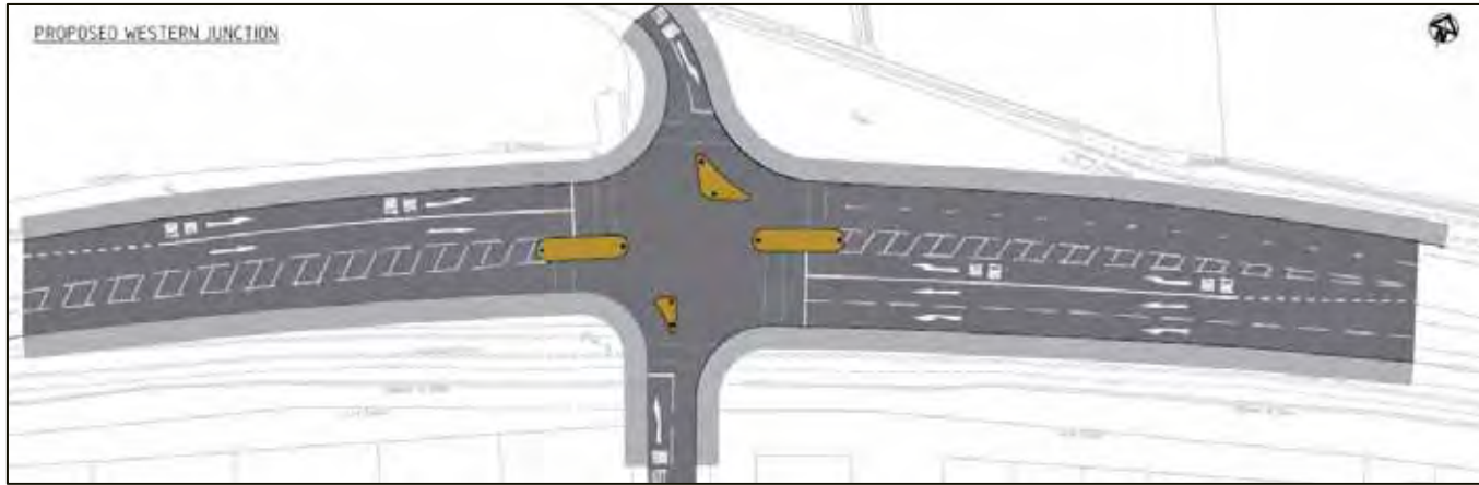
Fig 25 – Western junction – indicative left-in/left-out solution
