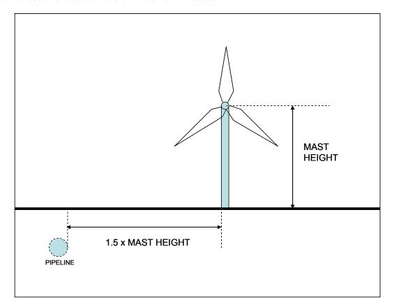
Based on the study, the recommended distance from the nearest part of the mast of the wind turbine at ground level mast to the nearest part of the pipeline has been identified as a minimum of 1.5 times the turbine mast height. The mast height is defined as the height from the ground level up to the centre line of the wind turbine axle.
